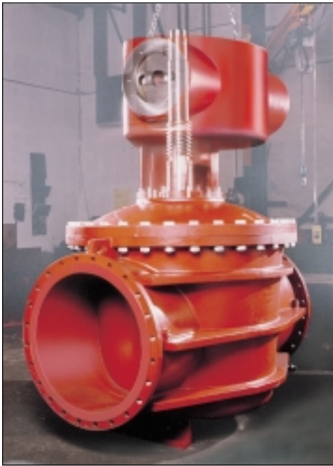
Mounting of the gearbox on top of the body.
