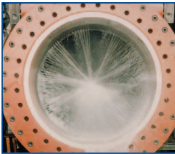
Water jets striking each other instead of the valve walls
