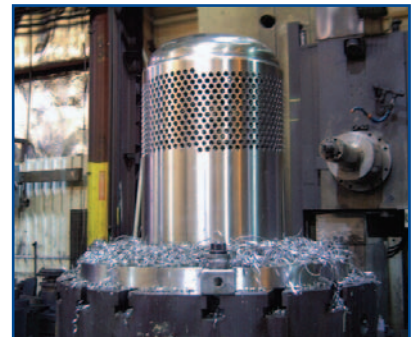
Nozzle pattern on the valve sleeve
